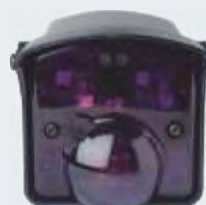
Radar / presence detector Comfort Radar movement and presence detection with infrared detection, fast and targeted automatic door opening, reliable advance protection, up to a height of max. 6 m, in areas with high levels of humidity and in outside areas, only the radar function is available, housing: protection category IP 65
